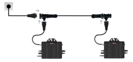
C. Then connect the AC plug cable to the local power grid.
