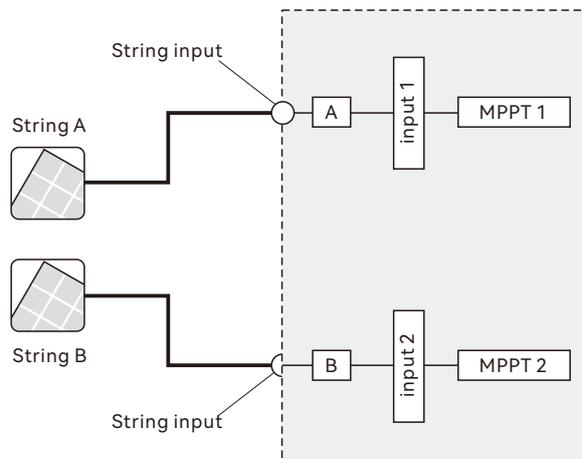
There are two MPPT's on the unit, so you can connect two independent MPPT channels.
