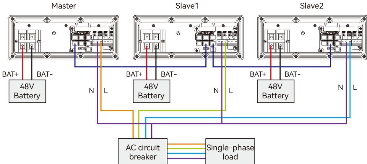
After connecting the power and communication cables, you will need to configure the master and slave settings, enable the group three-phase function, set the communication address, and phase sequence. Follow the steps below to configure these settings (requires monitoring server access).
