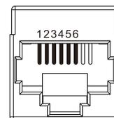
When the inverter receives an order from DRM0 connection, it will respond accordingly by reducing the output power to 0 ( by shorting the connection between RJ45 No.5 and No. ).
