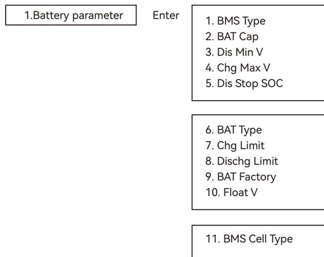
**a. BMS Type:** Battery charging and discharging maximum current mode(0: Default 1: Battery Control Maximum Charging Current; 2: Battery Control Maximum Charging and Discharging Current).
